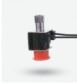
16075 24 VAC 3-Way In Rush Current: 0.45 A (10.8 VA) Holding Current: 0.30 A (7.2 VA) Compatible with: 3100
